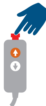
Image 6 Activation of emergency stops.
