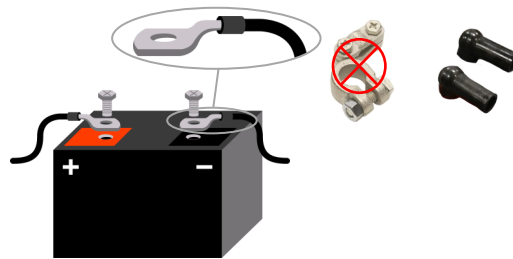
Figure 19. Fit the cable lug to the battery terminal (positive terminal first), without the terminal clamp. Make sure the cable lug is attached in the right direction. Use the new terminal protectors.
